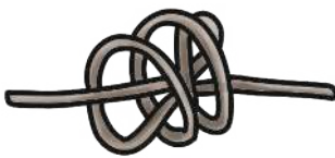
heaving line knot
