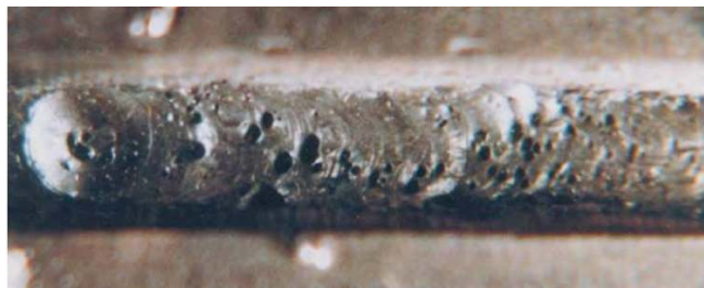
Gambar 8.11 Cacat porositas Sumber: American Welding Society 2015
