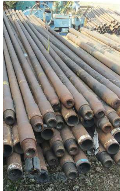
Gambar 6.20 Drill Pipe Sumber: Yudanto (2020)
