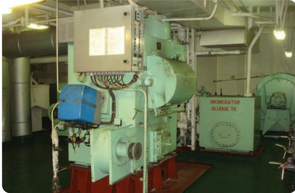
Gambar 9.26 Insinerator Kapal Sumber: Rajeev Jassal/myseatime.com (2017)
