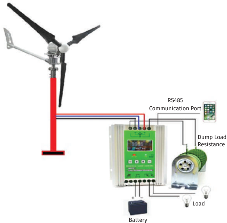
Gambar 3.58 Peralatan Control Charging System Pengisian Baterai
